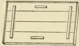
Under side of zinc top, showing cleats
